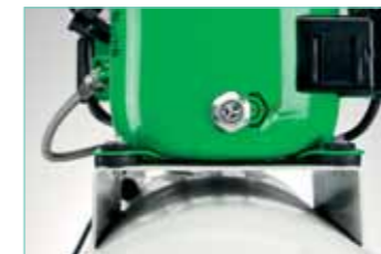
Clearview Oil Level Check
